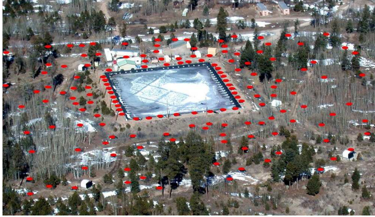
Figure 2.5: The Milagro detector: the pond with the positions of outriggers.
