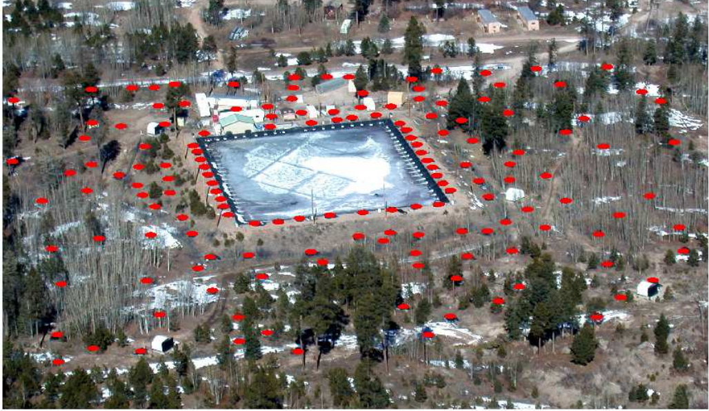
Figure 3.1: An aerial view of the Milagro detector. The pond is visible in the center of the photo. The red circles mark locations of the outrigger tanks.
